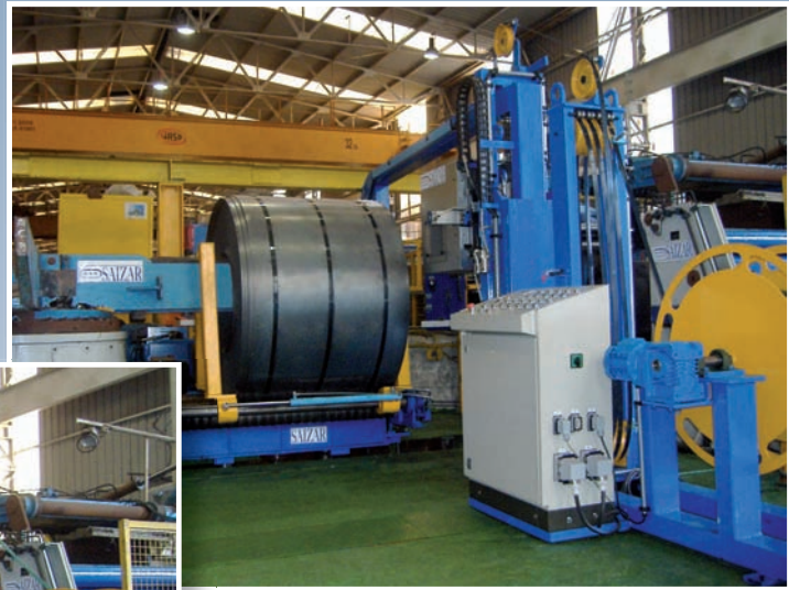
Coil circumferentially strapped by the automatic strapping machine with 32mm steel strap.
