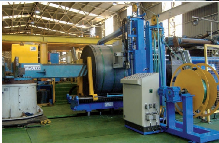
Strapping machine for the 32mm polyester strapping of cold coils
