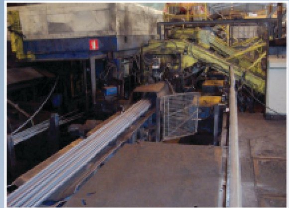
3 Rod binding machines do the binding of packages.
