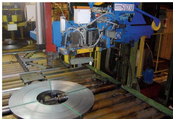
TITAN strapping machine for the radial strapping of coils with SAIZAR CASP-19 head for 19mm polyester strap.
