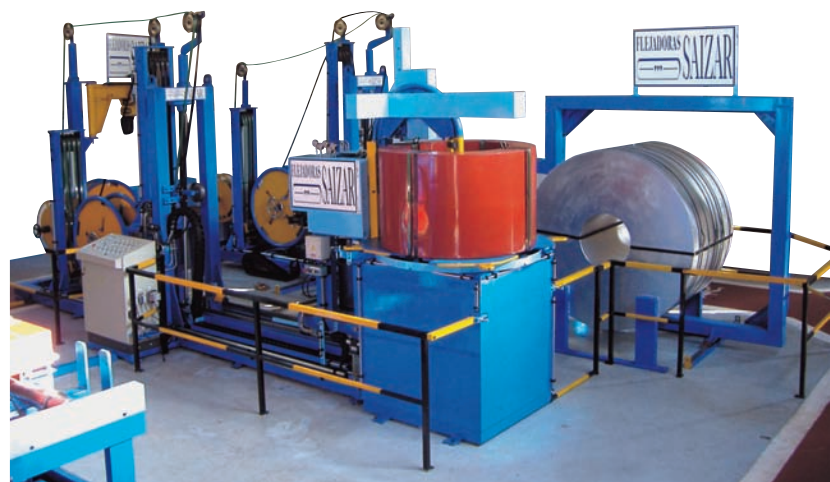
Automatic strapping machines for the circumferential and radial strapping of coils (with rings incorporation) with steel and polyester strap.
