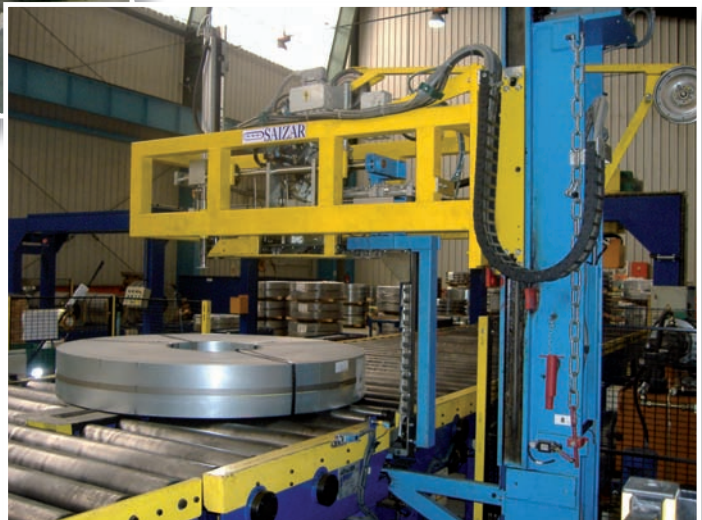
Strapping machine for the radial strapping of coils with 19mm steel strap
