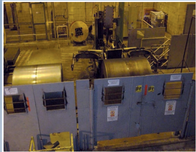
Strapping machine for the radial strapping of hot strip coils with 32mm steel strap.
