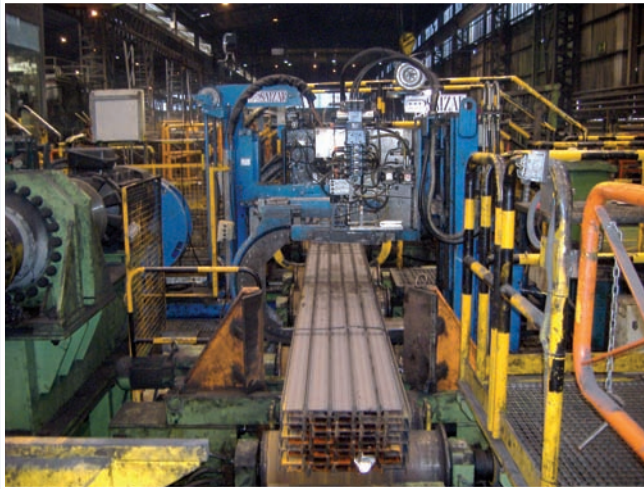
General view of two automatic strapping machines for the transversal strapping of profiles packages, with 32mm steel strap.
