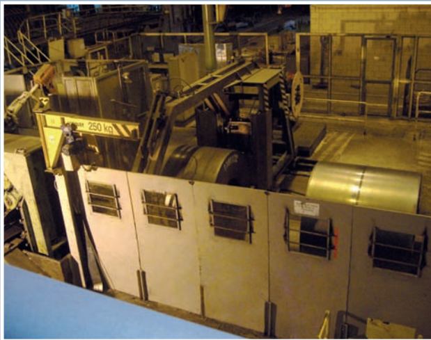
Strapping machine for the circumferential strapping of hot strip coils with 32mm steel strap.
