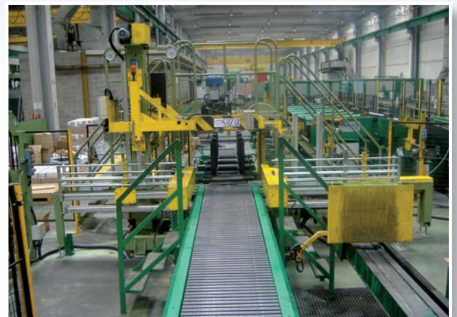
Strapping machine for the 32mm steel transversal strapping of tubes packages, with incorporation of wooden bars in automatic mode.
